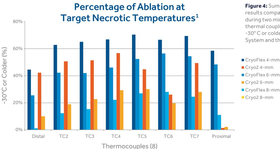
**Figure 4:** Summary of the in vitro testing results comparing the percentage of time during two minute ablations that each thermal couple recorded temperatures of -30° C or colder on the Medtronic CryoFlex System and the AtriCure cryoICE System.
