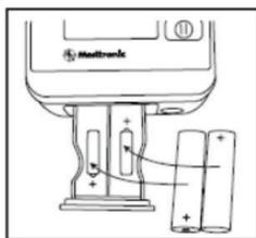
4. Close the battery drawer firmly until the battery drawer is fully latched.
