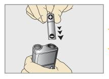
**Step 1.** Place the battery into the battery compartment with the negative (flat) end going in first.
