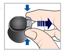
Remove the disconnect cover (the small plug below the button) by gently squeezing the sides of the disconnect cover then pulling it away from the insertion device.
