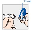
Twist plunger counter-clockwise to loosen and remove.
