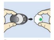
Remove transmitter from the charger to put it into 'search mode'.
