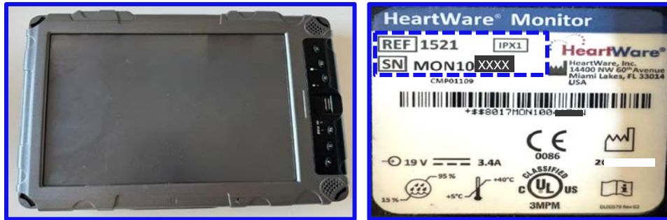
Figure 2. Identification of 'Xplortech' monitors. LEFT: gray monitor color; RIGHT: device label with model (REF) and serial number (SN).
