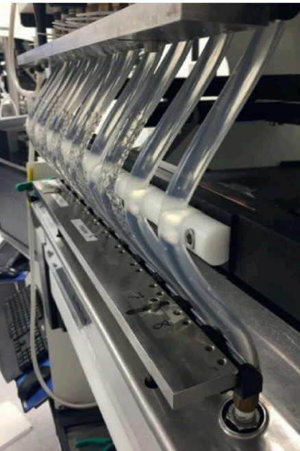
Fig. 1. MAPS testing equipment setup to simulate bending caused by hip flexion
