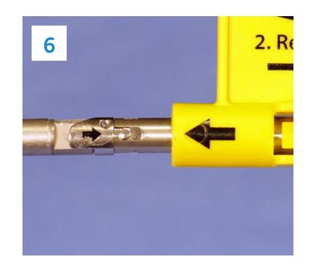
Ensure that the arrow on the shaft aligns with the shipping wedge arrow. Push the reload onto the distal end of the shaft until the two arrows meet.
