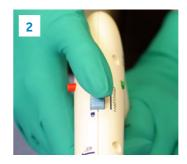
Pull and hold the blue lock switch button in the back position.
