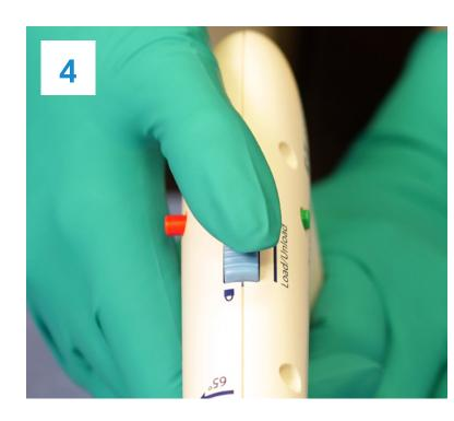
Pull and hold the blue lock switch button in the back position.
