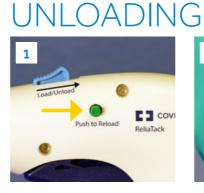
Push the green load button to expose the red portion of the toggle button and ensure the device is in the straight position.
