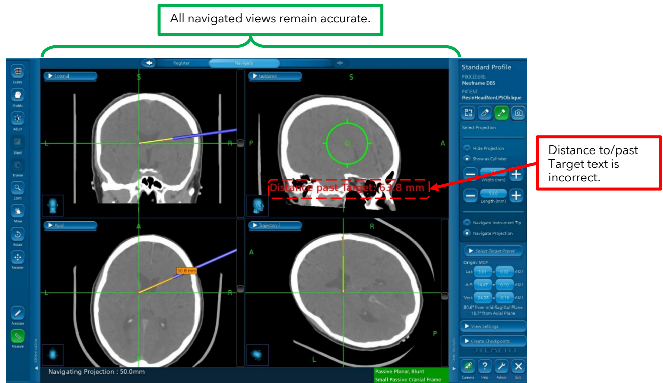
Figure 3 Distance to/past Target Text Inaccuracy seen in Navigate Task of NexFrame™ DBS
